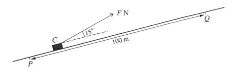
A crate C is pulled at constant speed up a straight inclined path by a constant force of magnitude F N, acting upwards at an angle of 15° to the path. C passes through points P and Q which are 100 m apart (see diagram). As C travels from P to Q the work done against the resistance to C's motion is 900 J, and the gain in C's potential energy is 2100 J. Write down the work done by the pulling force as C travels from P to Q, and hence find the value of F.
