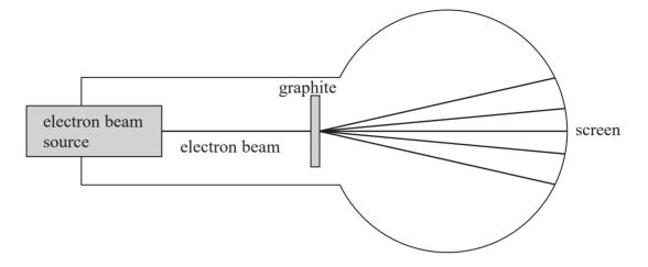
The diffraction pattern seen on the curved screen is shown below.
