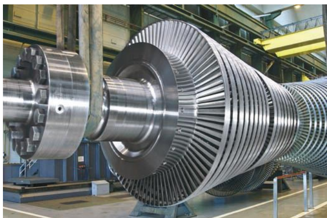
Figure 15.6 The rotor of a steam turbine
