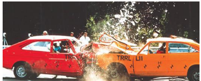
Figure 14.6 Cars in an impact test showing the collapse of the front crumple zone
