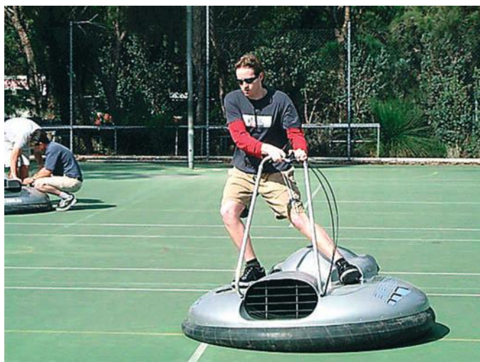
Figure 8.1 Friction is much reduced for an airboard.
