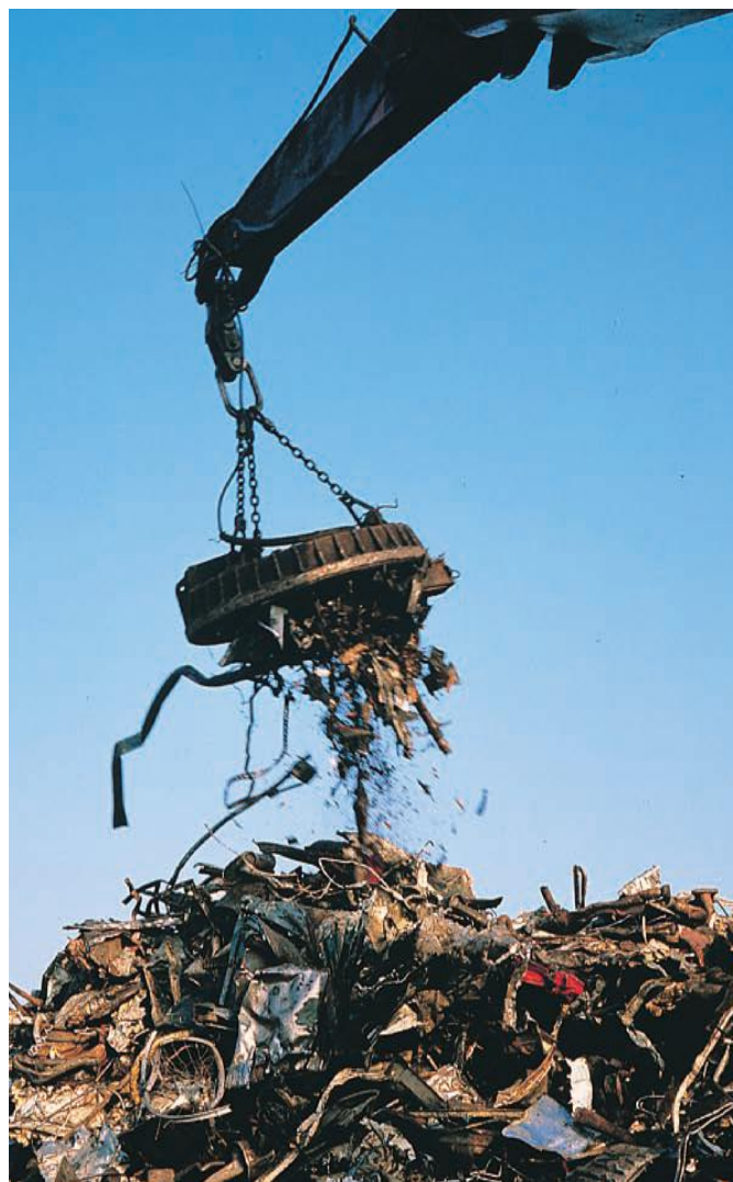
Figure 45.7 Electromagnet being used to lift scrap metal
