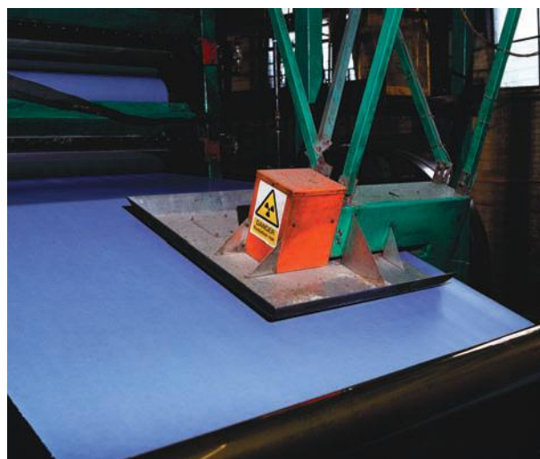
Figure 49.11 Quality control in the manufacture of paper using a radioactive gauge
