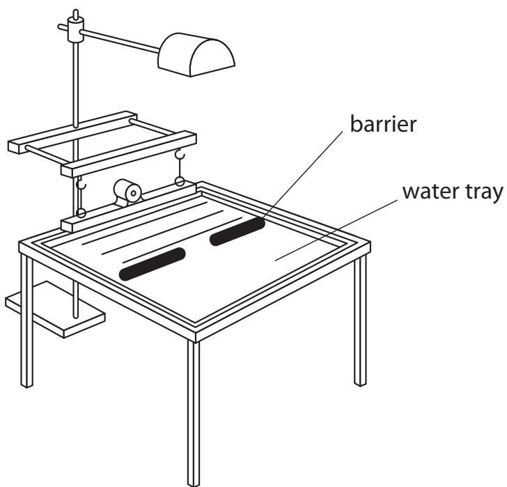
The ripple tank produces plane waves.
