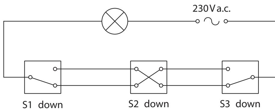
When all three switches are up, the lamp is on.
