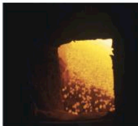
Figure 14.6 Limestone being heated in a lime kiln to produce quicklime (calcium oxide).
