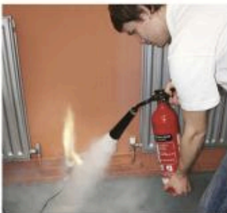
Figure 7.13 Using a carbon dioxide fire extinguisher to put out an electrical fire.
