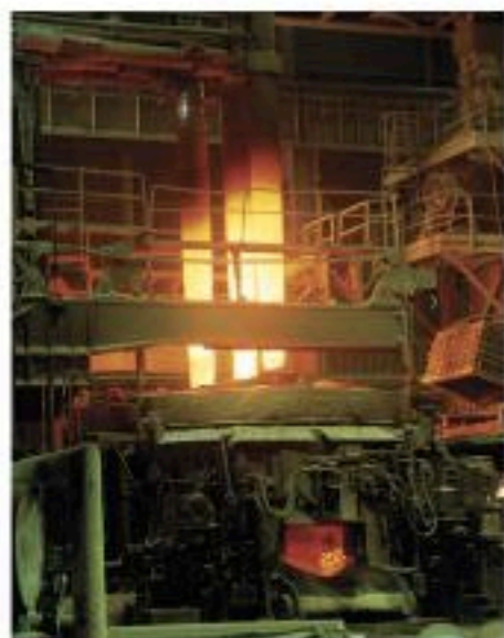
Figure 4.21 Three graphite electrodes glow red hot after their removal from an electric arc furnace used to produce steel
