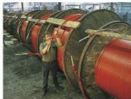
Figure 21.11 PVC is used to insulate electric cables.
