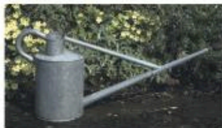
Figure 17.20 Galvanised iron doesn't rust even in constant contact with air and water.
