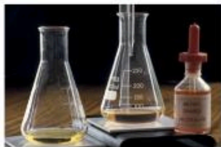
Figure 26.3 The end point colour for methyl orange – the flask on the left shows the colour before the end point.
