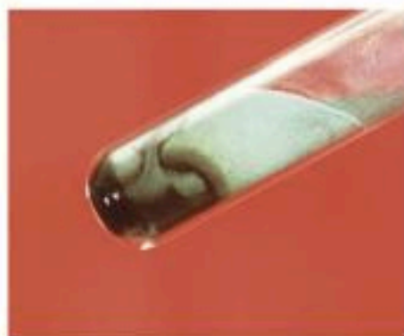
Figure 14.5 Copper(II) carbonate turns black on heating.
