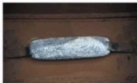
Figure 17.21 A sacrificial anode attached to a boat.
