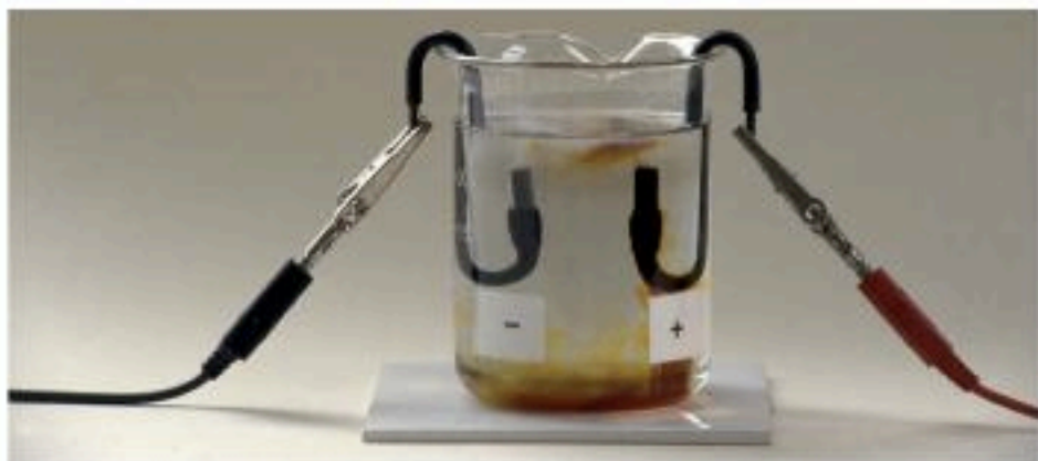
Figure 13.1 Part of an electric circuit involving the electrolysis of potassium iodide solution.
