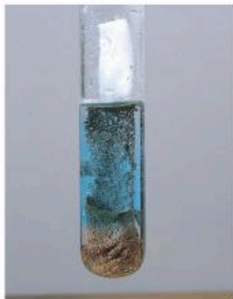
Figure 8.8 Zinc displaces copper from copper(II) sulfate solution.
