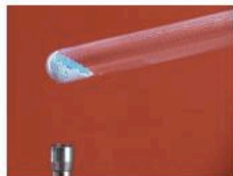
Figure 15.1 Copper(II) sulfate crystals are split into anhydrous copper(II) sulfate and water on gentle heating.
