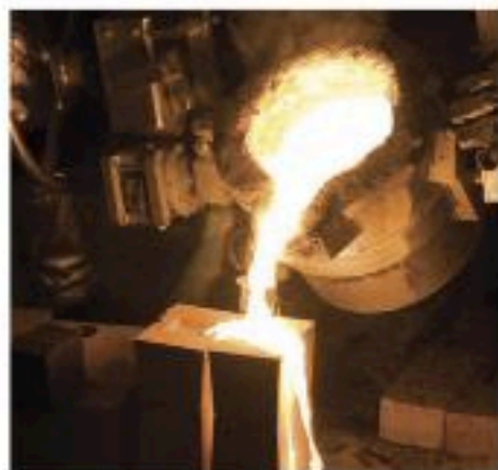
Figure 23.2 Molten lead tapped from the bottom of a furnace.
