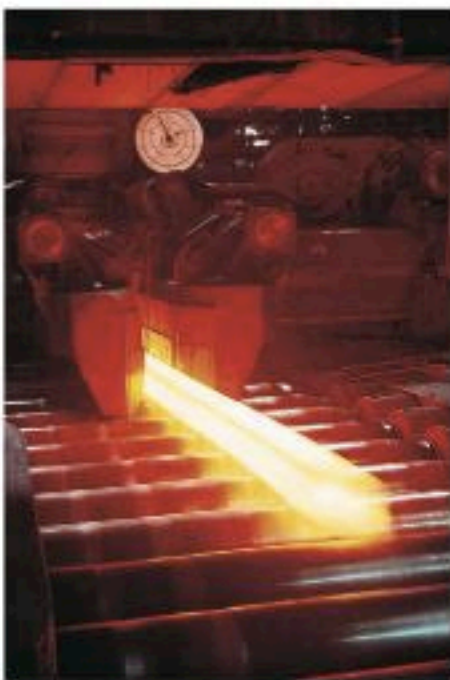
Figure 4.8 Steel being rolled into strips.
