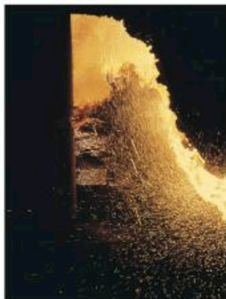
Figure 17.14 Molten iron being tapped from a blast furnace.
