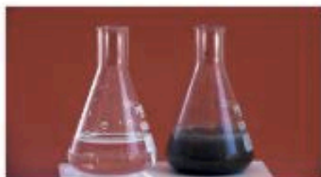
Figure 6.22 The flasks both contain hydrogen peroxide solution, the right-hand one has a little \text{MnO}_2 added to speed up oxygen production.
