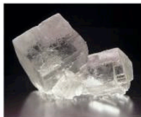
Figure 4.13 The shape of the sodium chloride crystal reflects the arrangement of the ions.
