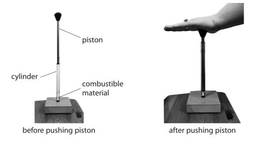
A small piece of combustible material is placed at the bottom of the cylinder.
