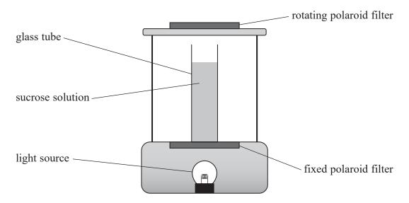
The angle of rotation depends on the concentration of the sucrose solution
