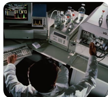
▲ A mass spectrometer, for finding relative molecular mass. It compares the mass of a molecule with the mass of a carbon-12 atom, using an electric field.
