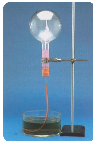
▲ The fountain experiment . The flask contains ammonia. It dissolves in the first drops of water that reach the top of the tube, so a fountain of water rushes up to fill the vacuum. (Any very soluble gas will show this effect.)
