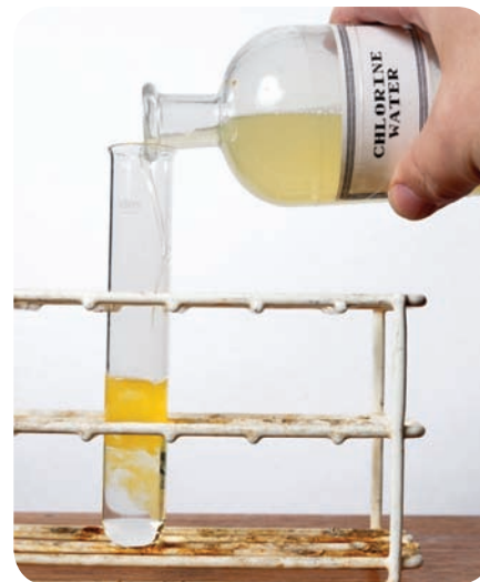
▲ Chlorine displacing bromine from aqueous potassium bromide.
