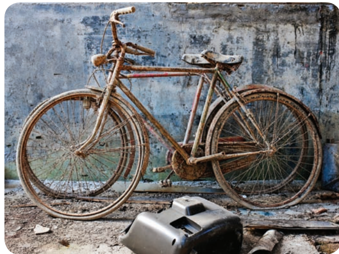
▲ And here, iron is being oxidised to iron(III) oxide again! We call this process rusting . It is ruining the bikes. The formula for rust is \text{Fe}_2\text{O}_3 \cdot 2\text{H}_2\text{O} .
