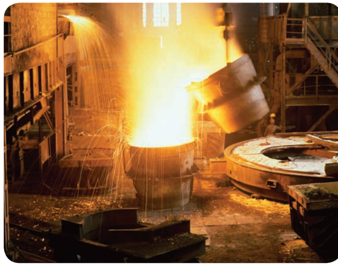
▲ Molten steel being poured out, in a steel works. Look how it glows. Temperature: around 1400°C.
