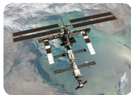
▲ Light metals such as aluminium and titanium are used in the International Space Station, 360 km above us.
