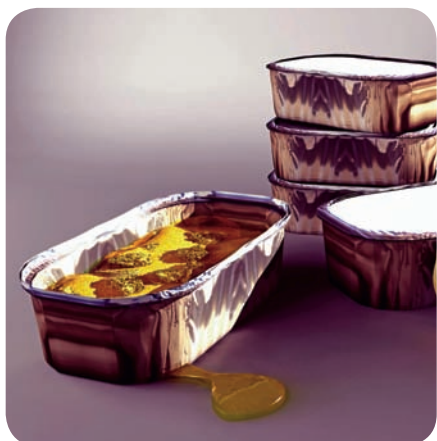
Aluminium foil is used for food cartons because it is non-toxic, resists corrosion, and can be rolled into thin sheets.
