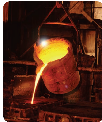
▲ Molten iron being poured out at an iron works. Hot – over 1540°C!
