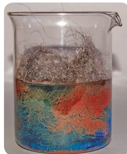
▲ Iron wool reacting with copper(II) sulfate solution. Iron is more reactive than copper so displaces the copper (deep pink) from solution.
