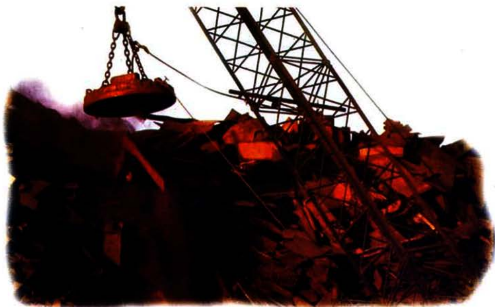
An industrial magnet attracts iron from waste materials.
