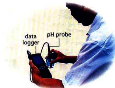
Fig. 11.13 Using a pH probe and a data logger to measure pH
