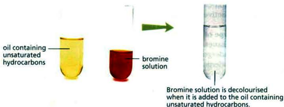
Fig. 23.5 Testing for the presence of unsaturated hydrocarbons
