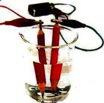
The lead in pencils contains graphite and can be used as inert electrodes in a simple set-up for electrolysis.
