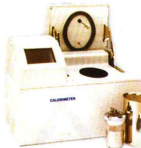
This apparatus is called a bomb calorimeter. It is used to determine the heat produced when a substance burns.
